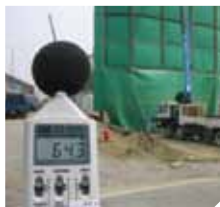
Measuring Noise Levels around the Construction Site
